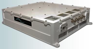
Wavestream's AeroStream Transceiver
