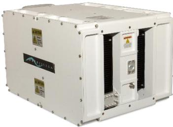
Wavestream has released an industry-leading Ka-band 160W Peak Envelope Power BUC for LEO/MEO gateway applications. The new BUC provides 65W of linear power. Leveraging Wavestream's patented Spatial advantEdge™ technology, this new gateway-focused BUC reaches power levels that could previously be achieved only by traveling wave tube amplifiers. Using the latest in GaN chips, Wavestream BUCs provide best-in-class performance with the smallest SWaP.
